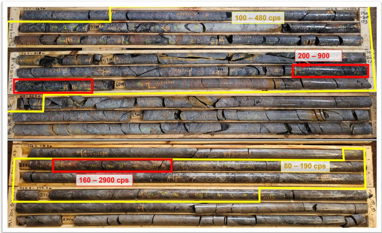
Figure 3: Two zones of typical reddish alteration and uranium mineralization intersected in ML-200.
