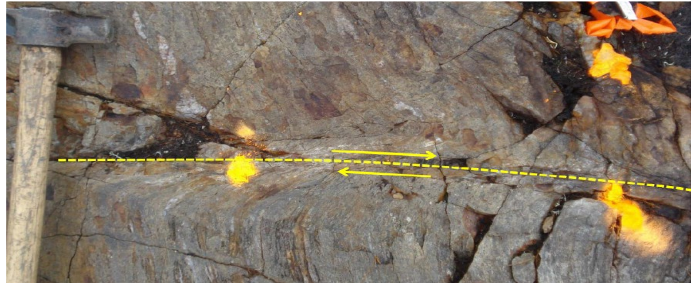
Uranium mineralization controlled by E/SE striking, steep-dipping, brittle ductile shears which transect earlier fabrics at Rumble Prospect
